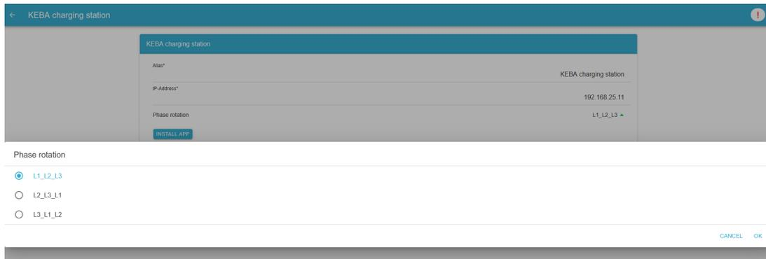
Figure 27. App installation — Phase rotation 2: Step 2
