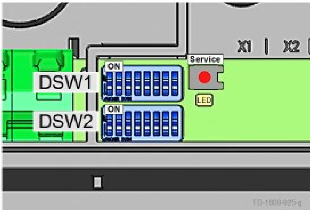
Figure 8. DIP switch DSW
