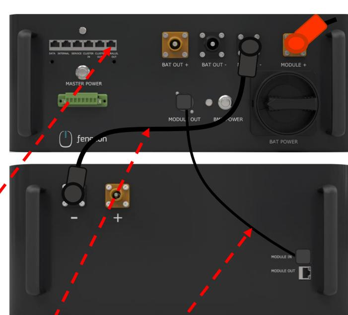
To the last battery module of the string connection „ - “
