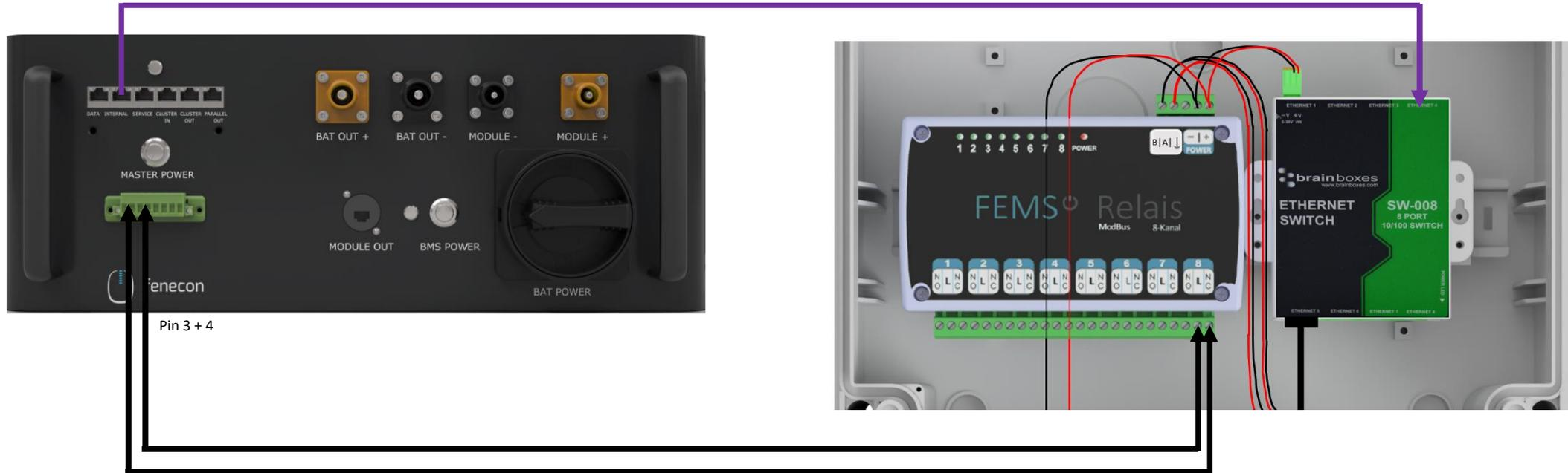
To the master BMS box - 8-pin connector: Pin 4 - Wire no. 1 of FEMS connection box Relay board connection 8 - Pin L
