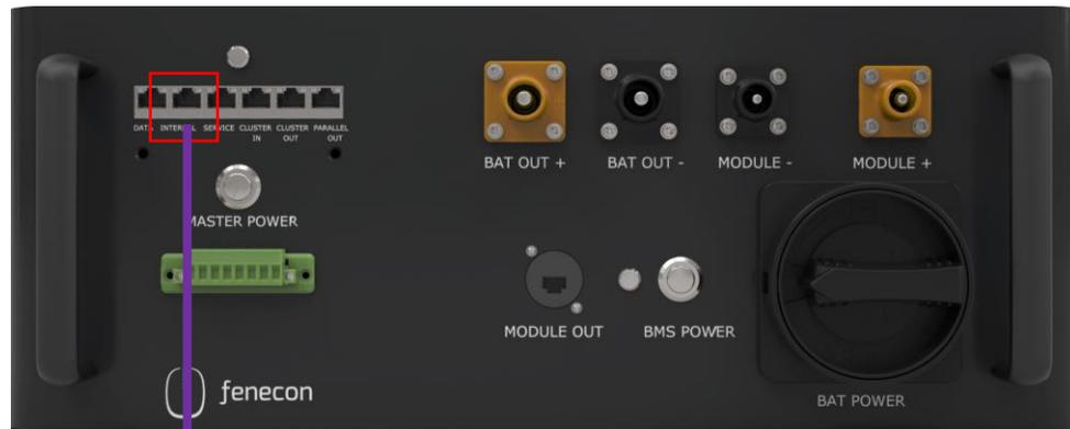
1. Pull the patch cable out of the "INTERNAL" connector on the master BMS
