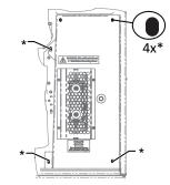
Fig. 17: Remove protective cover
