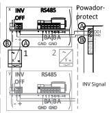
*Fig. 26:* Connect the device to Powador-protect
