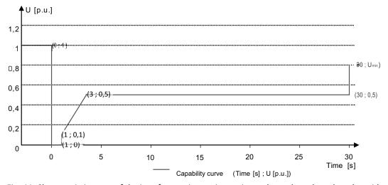
Fig. 44: Characteristic curve of the interference immunity against voltage drops based on the grid voltage
