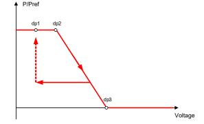
Fig. 36: Example characteristic curve without hysteresis
