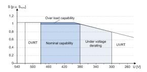
Fig. 30: Grid voltage-dependent apparent power for storage devices with  $U_N$  220/380, 230/400, 240/415 V
