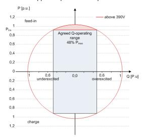
Fig. 49: P-Q operating range with limited active power (Qmax=Smax≠Pmax) Storage inverter
