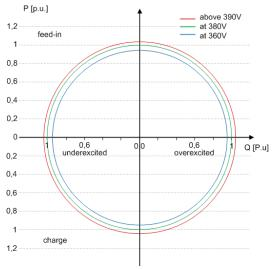
Fig. 29: P-Q operating range for storage devices with  $U_N$  220/380 V, 230/400 V, 240/415 V (Qmax=Smax)
