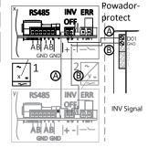
Fig. 27: Connect the device to Powador-protect
