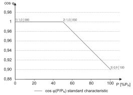
Fig. 31:  $\cos \phi$  / (P/Pn) standard characteristic curve with 3 nodes
