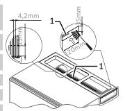
Fig. 52: Clean the cooling fins
