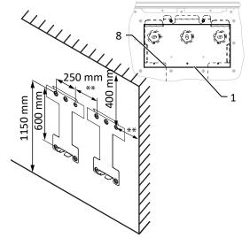
Fig. 11: Minimum clearances for wall mounting
