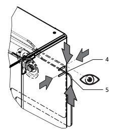
Fig. 13: Lift the device using the opening
