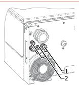
Fig. 24: Insert the Ethernet cable
