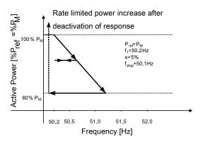
Fig. 42: Example behaviour with hysteresis (mode 1)
