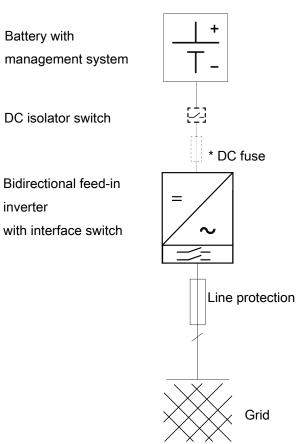
Fig. 4: Circuit diagram for a system with one bidirectional feed-in inverter
