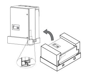
Fig. 10: Setting the device upright
