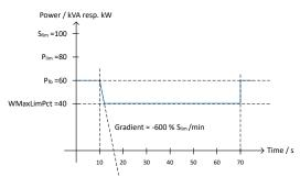
Fig. 33: Power gradient according to sample parameters and calculation
