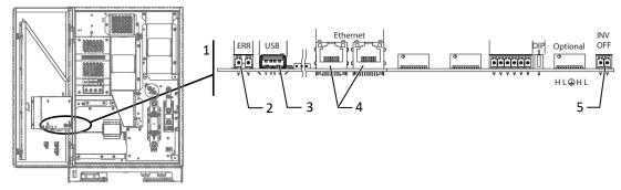
Fig. 23: Communication circuit board: Connection and assignment of the interfaces
