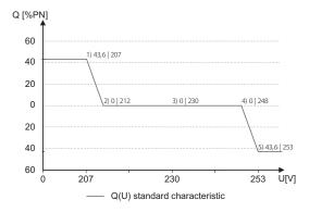
Fig. 32: Q(U) standard characteristic curve with 5 nodes
