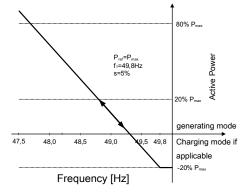
*Fig. 43:* Example behaviour without hysteresis (mode 2) At the time of activation, the inverter is in charging mode at 20% charging capacity.
