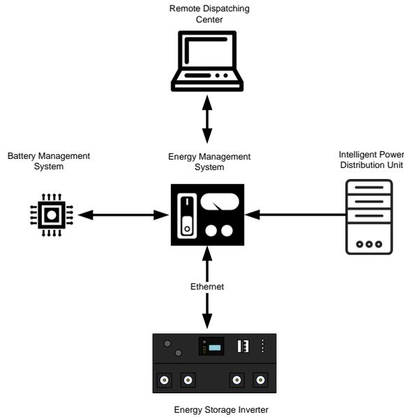
Fig. 5-2 Inverter connecting with EMS through Ethernet
