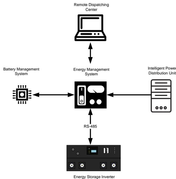
Fig. 5-1 Inverter connecting with EMS through RS-485
