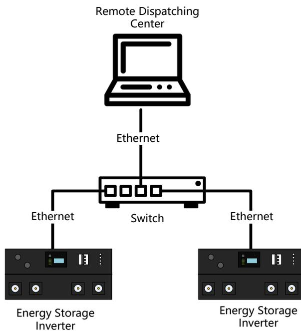
Fig. 5-4 Structure diagram for background monitoring system
