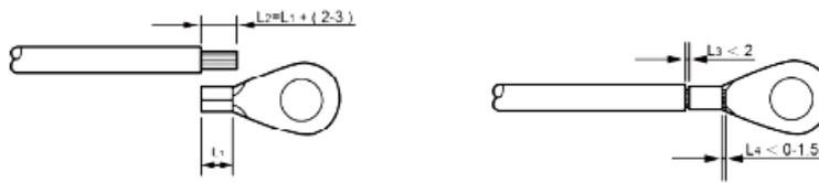
Fig. 3-5 Wiring stripping
