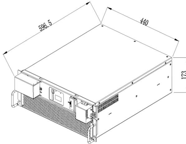
Fig. 2-2 Overall dimension of PWS2-30M-EX (unit: mm)
