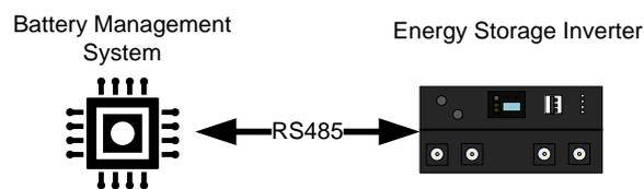
Fig. 5-3 Communication between PWS2-30M-EX and BMS
